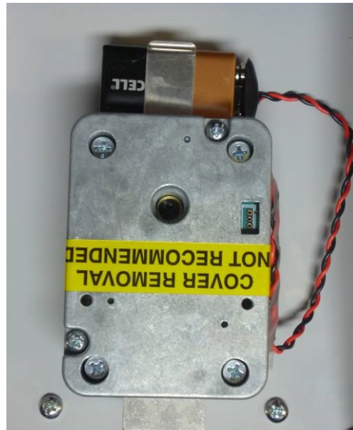
Figure 2 Battery Location and Replacement
